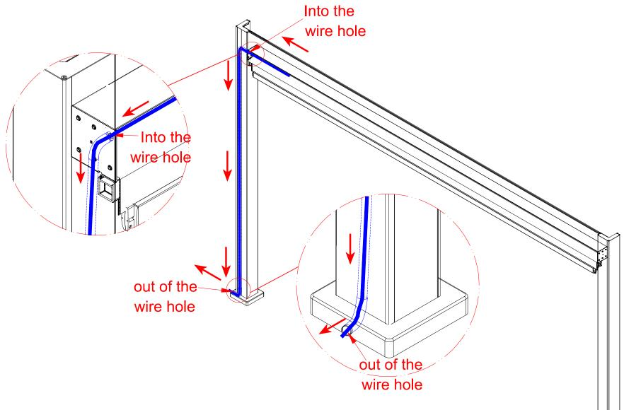
6.First, put the "wires guide" head through the outlet hole into the PVC pipe. And slide in and out through the inlet hole. The "wires guide" will be tied together with both ends of the wire. Then pull the "wire guide" from the outlet hole so that the wire enters the PVC pipe from the inlet hole as shown in the diagram, and comes out of the outlet hole along the PVC pipe.
